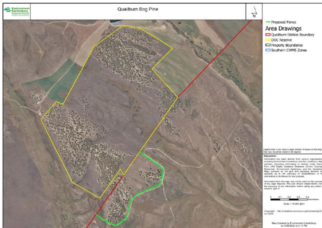
Figure 2. Proposed 7-wire sheep fence at Quailburn station to protect bog pine habitat.
